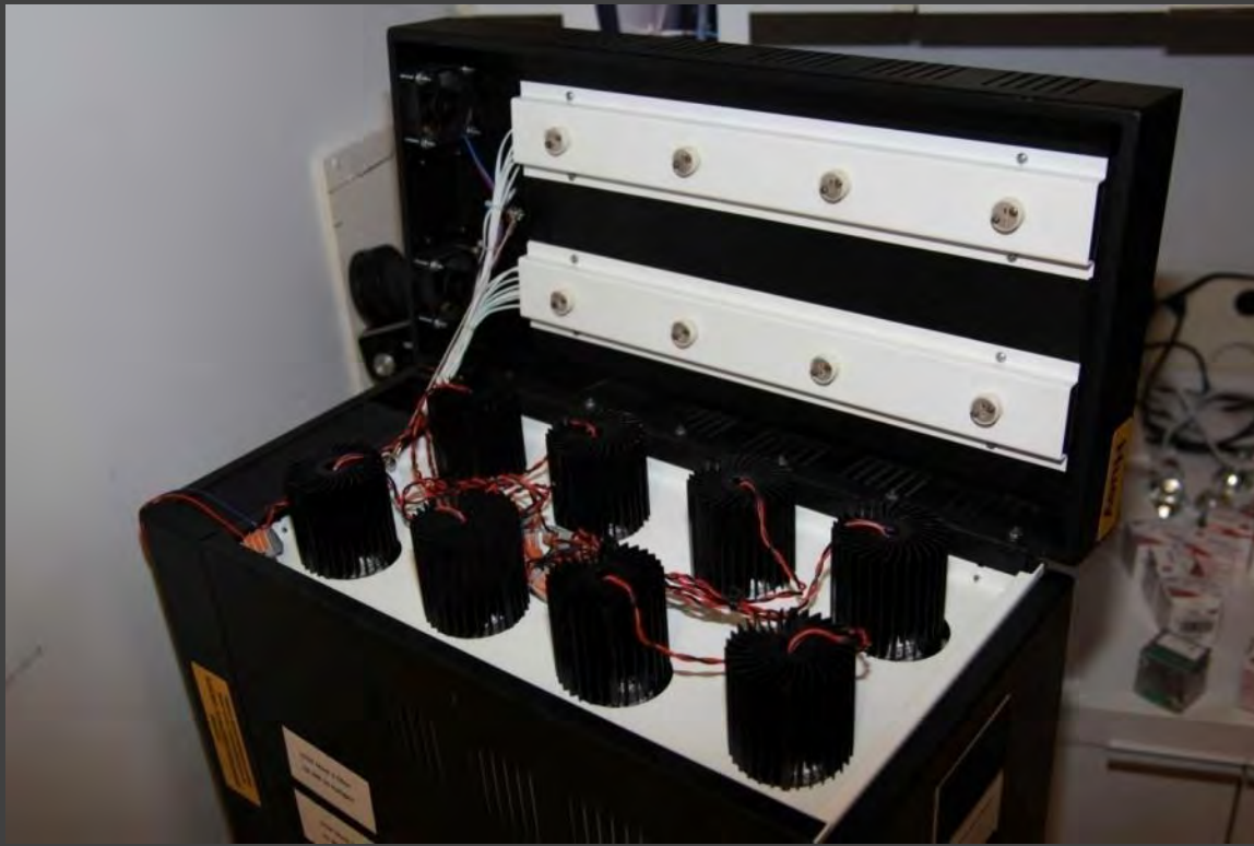
Xicato LED Light Engine Installed
