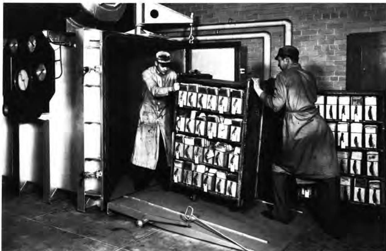
In this June 1936 photograph, employees of the Repair and Preservation Division wheel a cart of Veterans Administration files into a vacuum chamber for fumigation.
